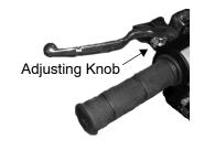
**NOTE:** The adjustment range is limited. Never apply excessive force to the knob. Always turn the knob manually.
